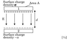
Fig. Capacitance of a parallel plate capacitor A parallel plate capacitor consists of two large plane parallel conducting plates separated by a small distance d. The two plates have charges q and -1 and distance between them is d.
