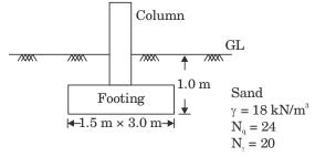
**9.** The net ultimate bearing capacity (kN/m2) of the footing based on Terzaghi's bearing capacity equation is
