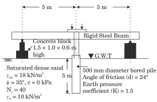
12. The maximum pressure that can be applied with a factor of safety of 3 through the concrete block, ensuring no bearing capacity failure in soil using
