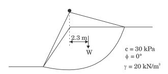
The length of the arc of the slip circle is 15.6 m and the area of soil within the slip circle is  $82 \text{ m}^2$ . The radius of the slip circles is 10.3 m. The factor of safety against the slip circle failure is nearly equal to
