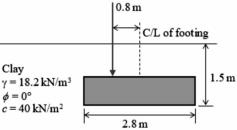
Using Meyerhoff's method, the load (in kN, round off to two decimal places) that can be applied on the footing with a factor of safety of 2.5 is \_\_\_\_\_
