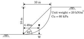
The factor of safety of the slope against slip failure, is
