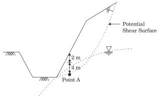
The soil exhibits c' = 20 kPA,  $\phi' = 18^{\circ}$ , and the undrained shear strength = 80 kPa. The unit weight of water is 9.81 kN/m<sup>3</sup>. The unit weights of the soil above and below the ground water table are 18 and 20 kN/m<sup>3</sup>, respectively. If the shear stress at point A is 50 kPa, the factors of safety against the shear failure at this point, considering the undrained and drained conditions, respectively, would be
