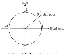
one zero at z = 1 & 2 zeros at  $z = \pm j$ 3 poles at z = 0Hence, option (c) is correct.
