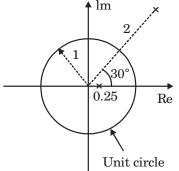
The ROC should encircle unit circle to make the system stable. From the given pole pattern it is clear that, to make the system stable, the ROC should be two-sided. Thus impulse response for the system should be two-sided.
