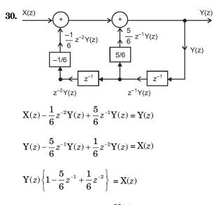
T.F. of the system, H(z) =  $\frac{Y(z)}{X(z)} = \frac{1}{\left(1 - \frac{5}{6}z^{-1} + \frac{1}{6}z^{-2}\right)}$  $H(z) = \frac{z^2}{\left(z^2 - \frac{5}{6}z + \frac{1}{6}\right)}$  $H(z) = \frac{z^2}{\left(z - \frac{1}{2}\right)\left(z - \frac{1}{3}\right)}$
