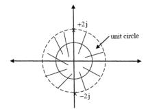
Thus ROC must be inside the circling radius 2. x[n] must be a non-causal signal.
